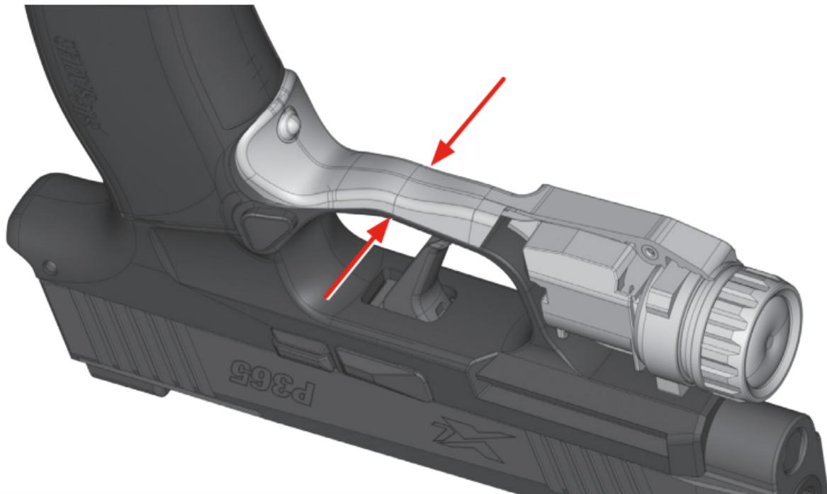
3. Insert tab of left housing (A) into right housing (B) at 30° angle. Mate left housing (A) to right housing (B).
